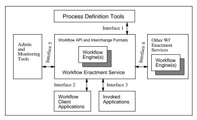
Fig. 4.1. WfMC Reference Model
