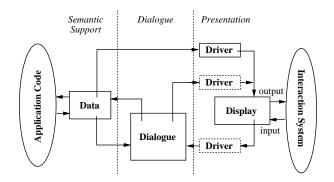
Figure 1: The 4D functional architecture
