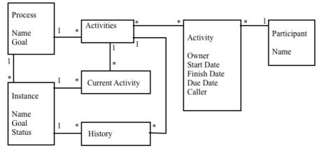
Figure 8 – Process model. We only show the elements necessary to understand basic functionality, which evolves around processes, activities and process instances.
