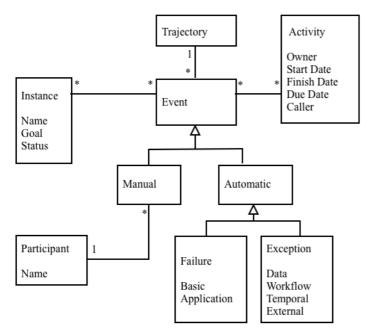
Figure 9 – Detection model, organized around hazard trajectories. A trajectory serves to organize and maintain the evolution of events according to chronological time. Note that hazards may be associated with specific process instances and activities.
